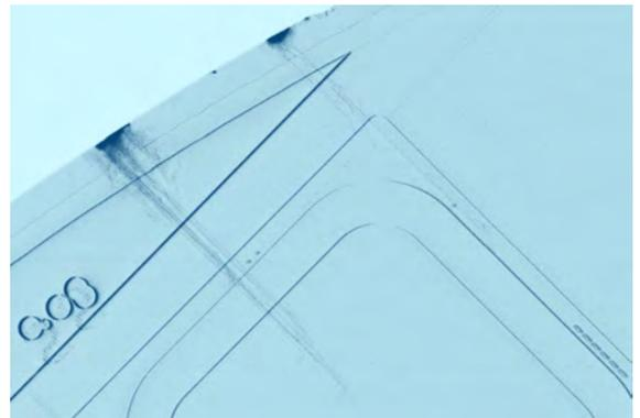
Fig. 4: Detailed X-ray transmission topogram of the 400 reflex for a specific area of an 200 mm Si wafer where glide-planes can be seen. (Photo: Fraunhofer IISB)
