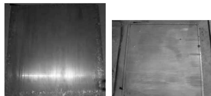
A company in China to produce silicon ingot of 840x840 mm<sup>2</sup> in cross-section using Jinggong's furnace: 120mm (left) and 60mm (right) from bottom
